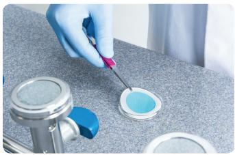
**Step 8**Filter support can easly be removed for decontamination.
